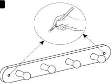
Mark mounting holes by placing the 3 in 1 on wall in position and use the pre - drilled holes in the sto -ve w/accessories to mark the drill locations on the wall.
